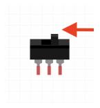
• Turn it off by pushing the switch from left to right
